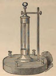
Fig. 63. Hydro-Rheostat (Galvano-Faradic Manufacturing Co.).
